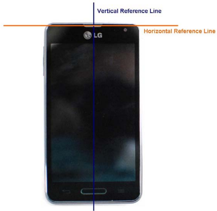
SAR Test Setup Photo 10: Vertical and Horizontal Reference Lines
