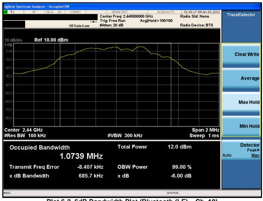
Plot 6-2. 6dB Bandwidth Plot (Bluetooth (LE) - Ch. 19)
