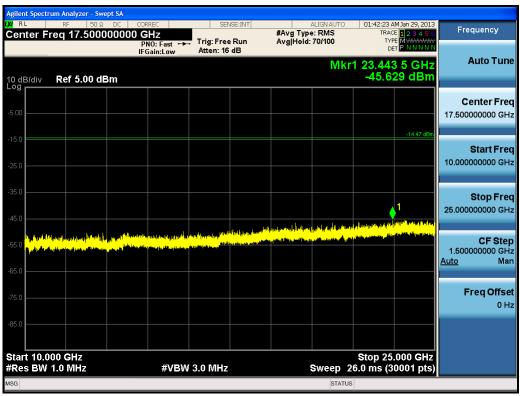
Plot 6-10. Conducted Spurious Plot (Bluetooth (LE) - Ch. 0)
