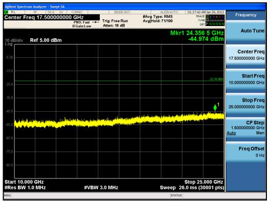
Plot 6-28. Conducted Spurious Plot (802.11b - Ch. 6)
