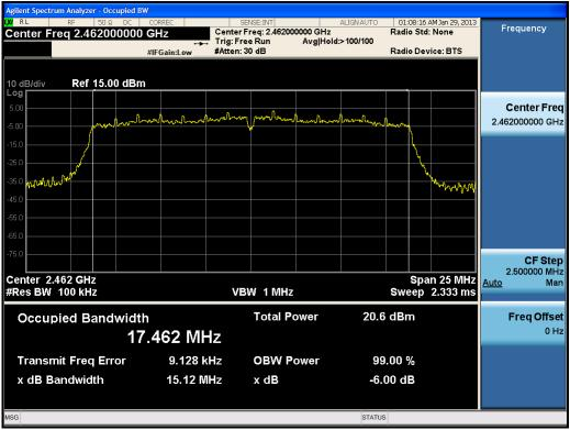
Plot 6-9. 6dB Bandwidth Plot (802.11n (2.4GHz) - Ch. 11)
