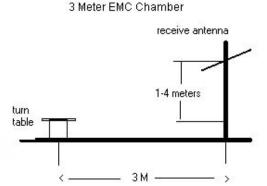
Figure 6-6. Test Instrument & Measurement Setup
