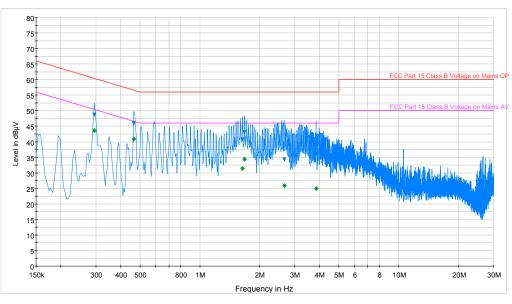
FCC Part 15 Class B Voltage on Mains AV.LimitLine Preview Result 1-PK+ FCC Part 15 Class B Voltage on Mains QP.LimitLine Final Result 1-QPK
