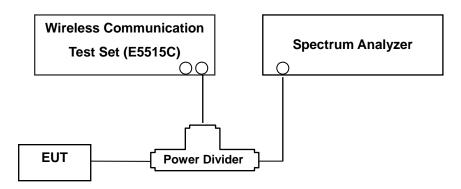
(Configuration of conducted Emission measurement) Test Procedure
