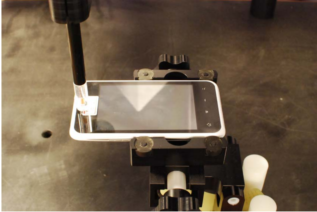
Figure 13-1 Test Setup for Wireless Device
