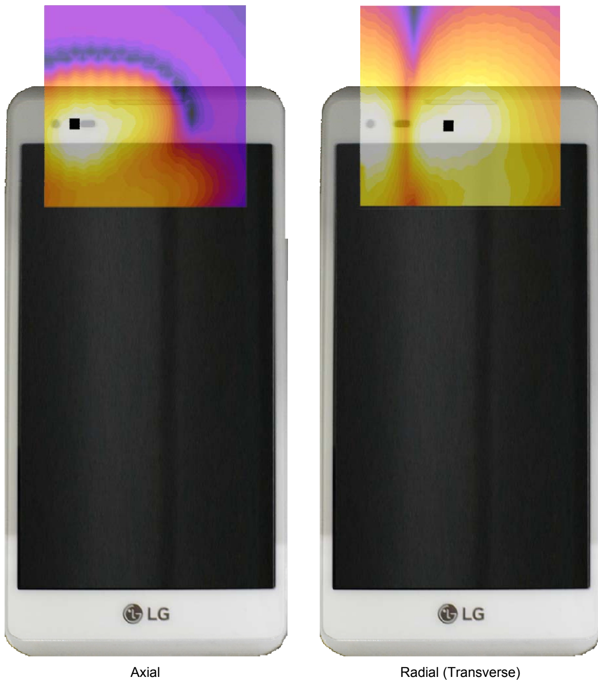
Figure 13-3 T-Coil Scan Overlay Magnetic Field Distributions
