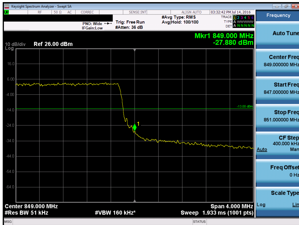
Plot 7-120. Upper Band Edge Plot (Band 5/26 – 5.0MHz QPSK – RB Size 25)
