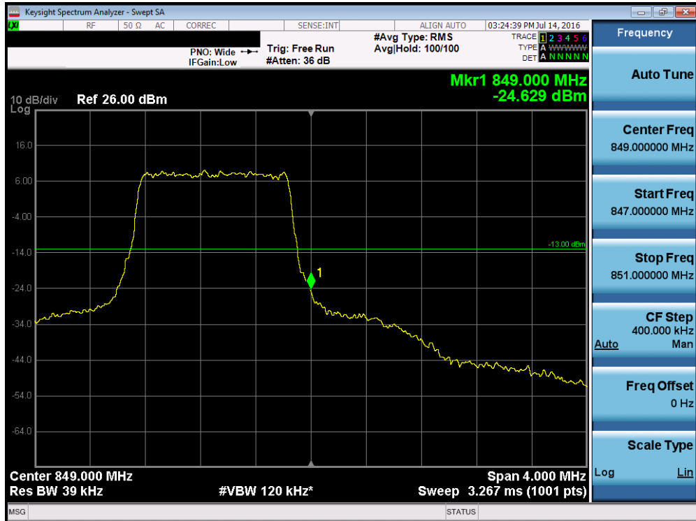
Plot 7-112. Upper Band Edge Plot (Band 5/26 – 1.4MHz QPSK – RB Size 6)
