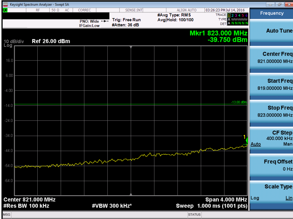
Plot 7-111. Lower Extended Band Edge Plot (Band 5/26 – 1.4MHz QPSK – RB Size 6)
