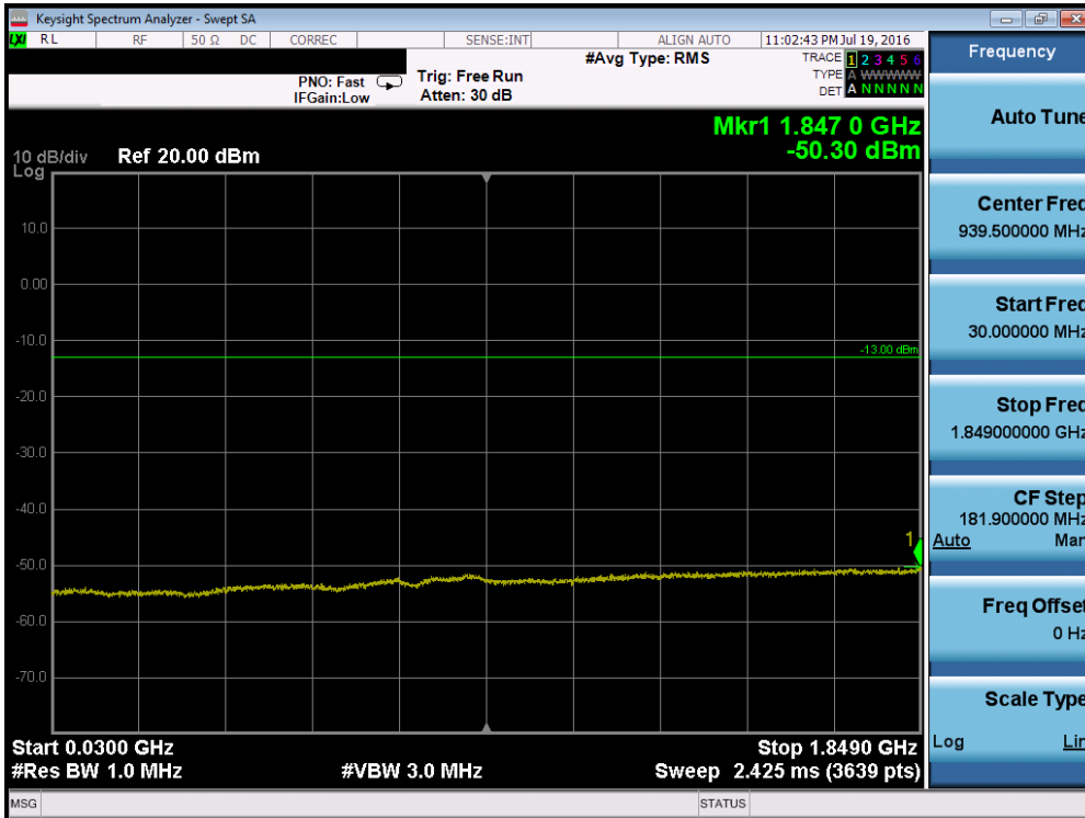
Plot 7-78. Conducted Spurious Plot (Band 2/25 – 20.0MHz QPSK – RB Size 1, RB Offset 0– Low Channel)
