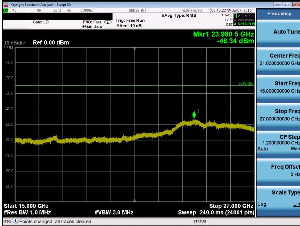
Plot 7-95. Conducted Spurious Plot (Band 41 – 5.0MHz QPSK – RB Size 1, RB Offset 0 – High Channel)
