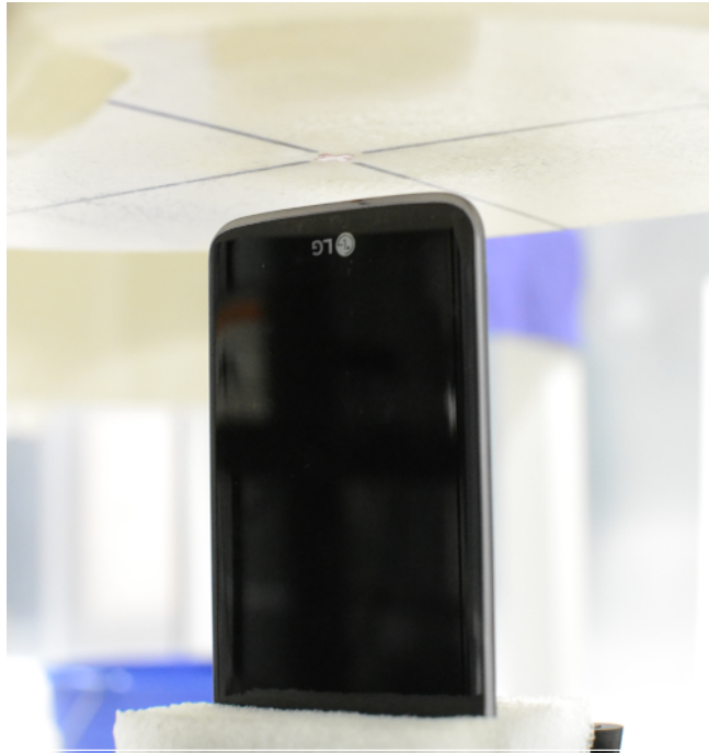
SAR Test Setup Photo 8 – Bottom Edge (10 mm)
