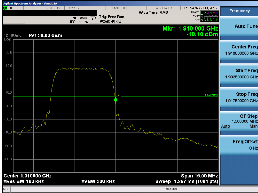
Plot 7-80. Band Edge Plot (PCS WCDMA Mode – Ch. 9538)
