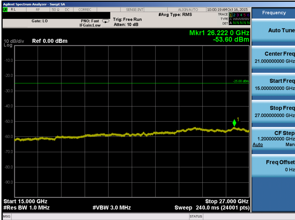
Plot 7-60. Conducted Spurious Plot (Band 41 – 10.0MHz QPSK – RB Size 1, RB Offset 0 – Low Channel)
