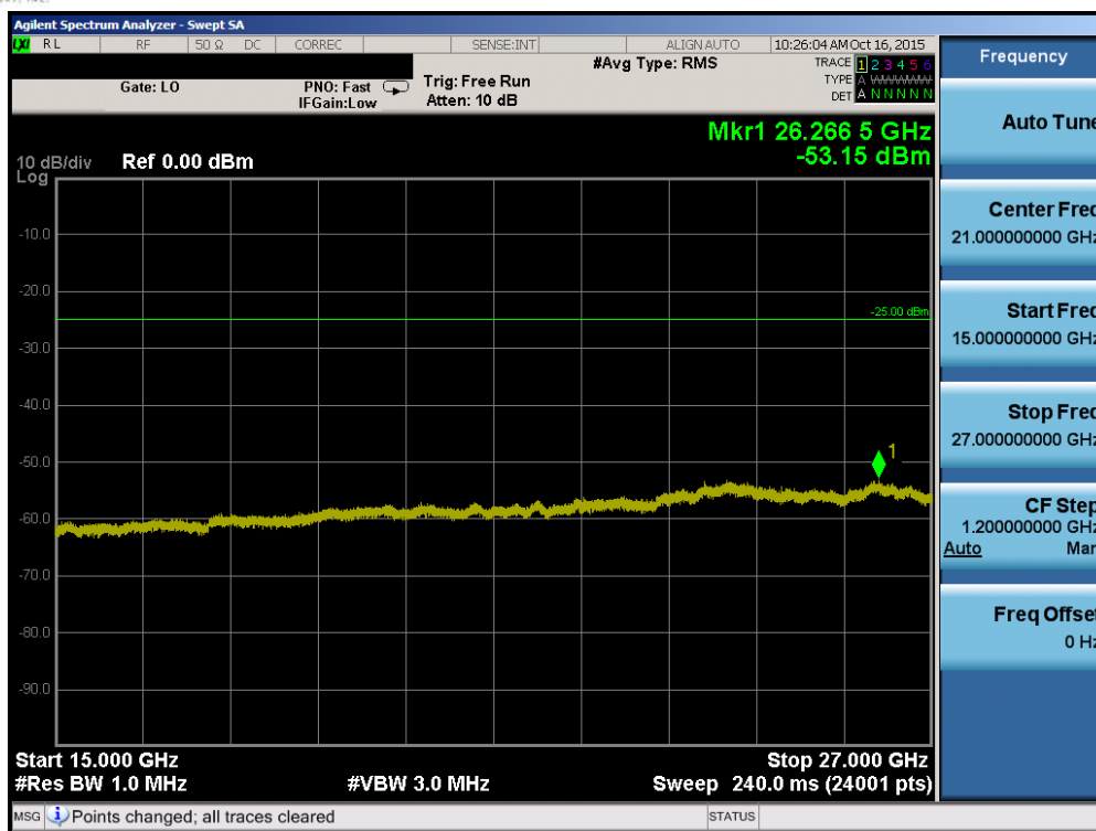
Plot 7-81. Conducted Spurious Plot (Band 41 – 20.0MHz QPSK – RB Size 1, RB Offset 0 – Mid Channel)
