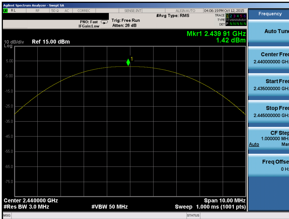
Plot 7-5. Peak Power Plot (Bluetooth (LE) – Ch. 19)
