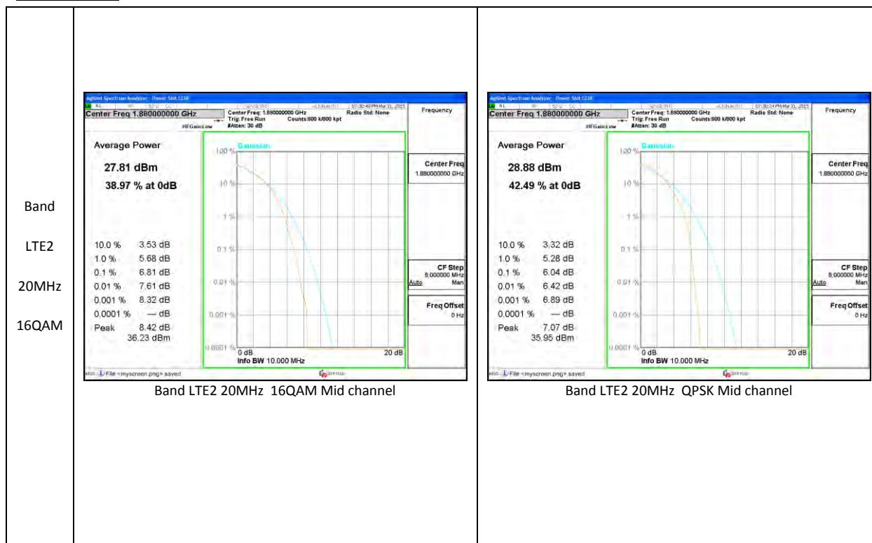
Band LTE2 20MHz 16QAM Mid channel
