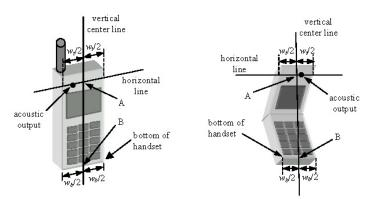
Figure 4-3 Handset Vertical Center & Horizontal Line Reference Points
