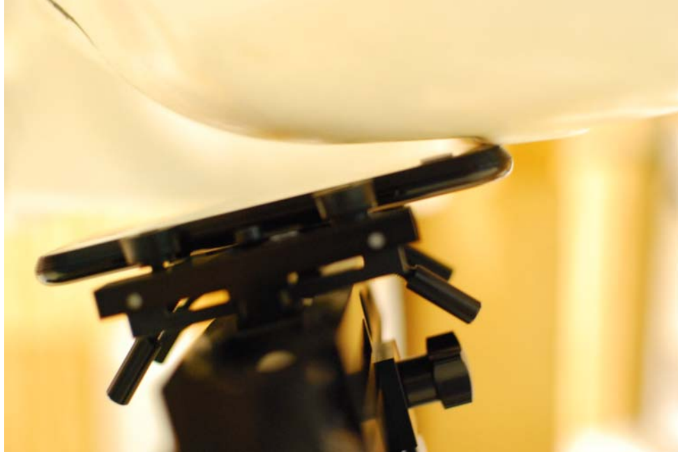
SAR Test Setup Photo 4 – Left Tilt
