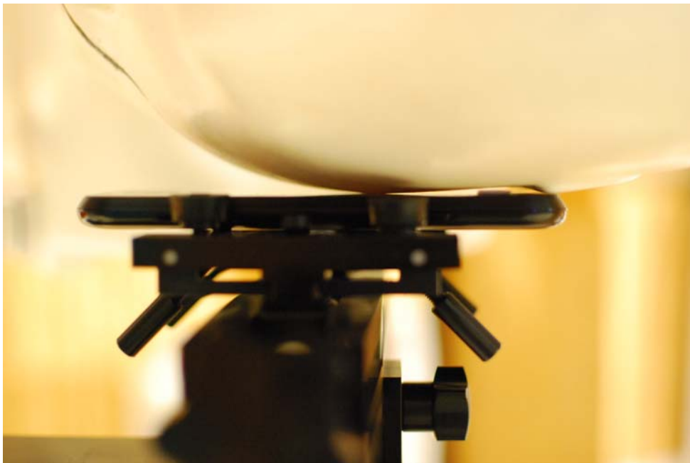
SAR Test Setup Photo 3 – Left Cheek
