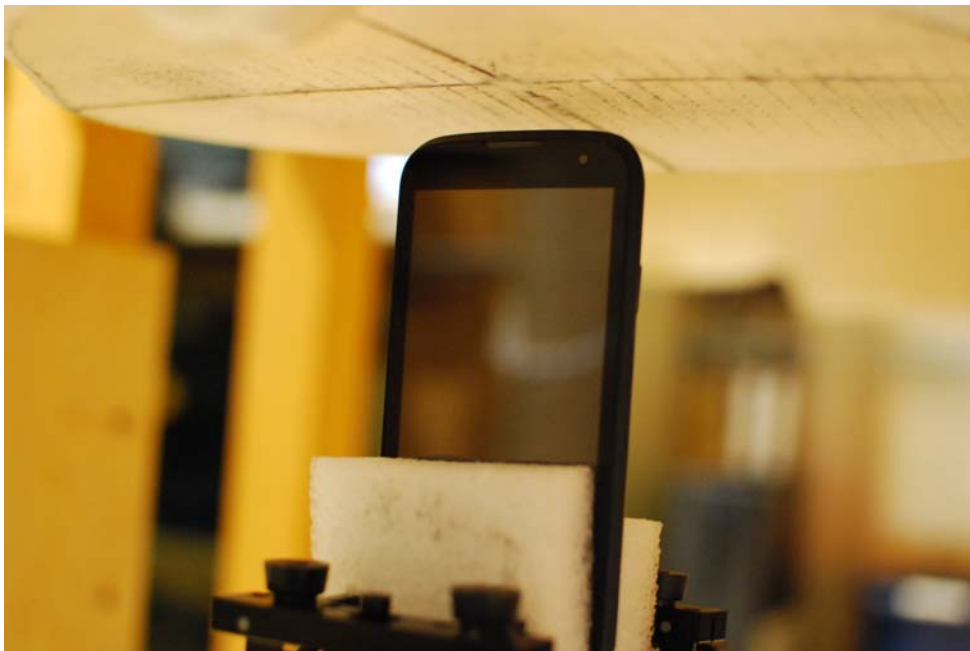
SAR Test Setup Photo 7: top at 1.0 cm
