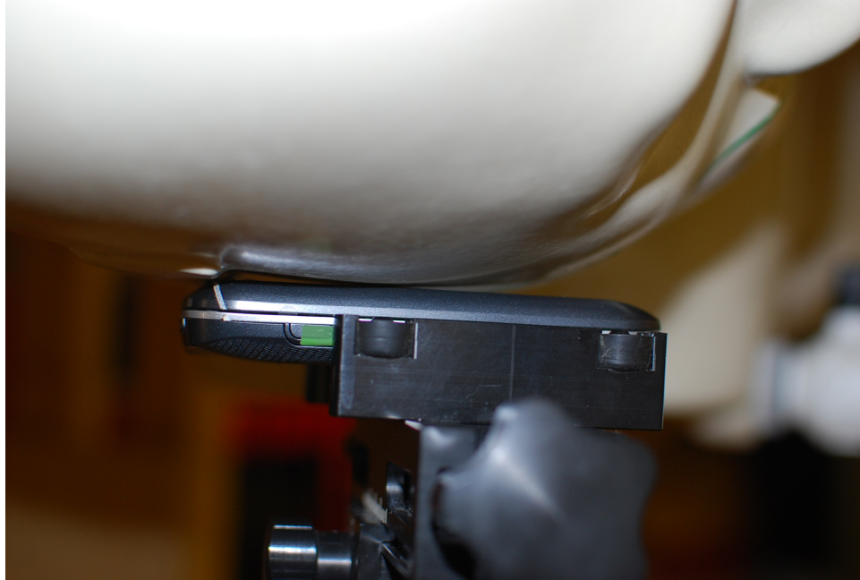
SAR Test Setup Photo 1 – Right Touch
