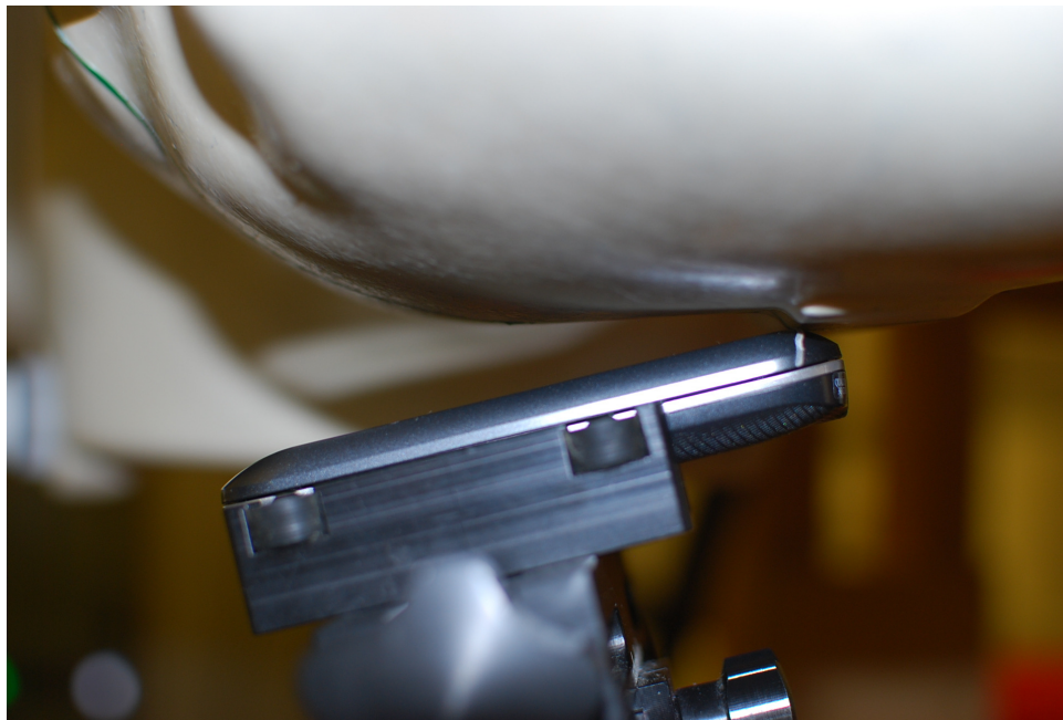
SAR Test Setup Photo 4 – Left Tilt
