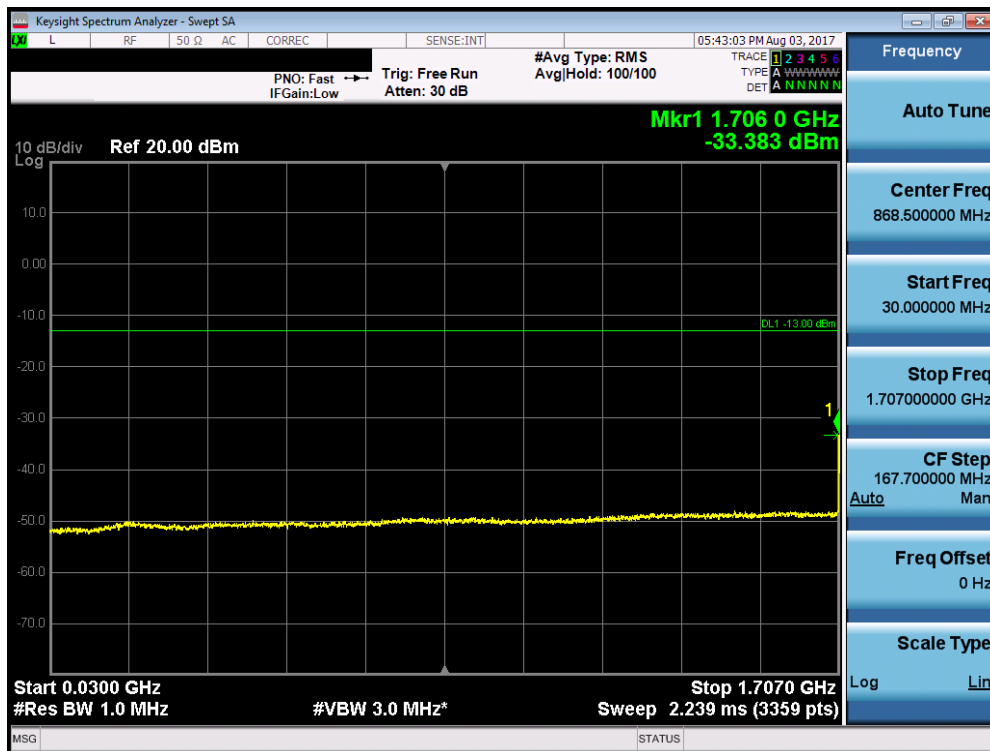
Plot 7-69. Conducted Spurious Plot (Band 4 – 3.0MHz QPSK – RB Size 1, RB Offset 0 – Low Channel)
