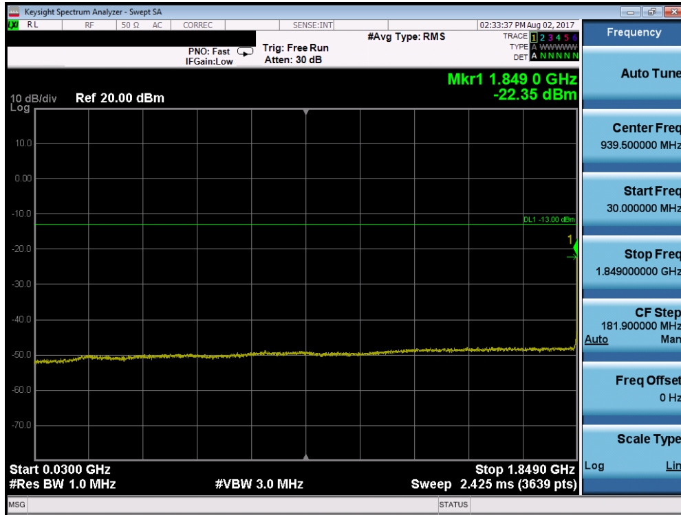
Plot 7-78. Conducted Spurious Plot (Band 2/25 – 15.0MHz QPSK – RB Size 1, RB Offset 0 – Low Channel)
