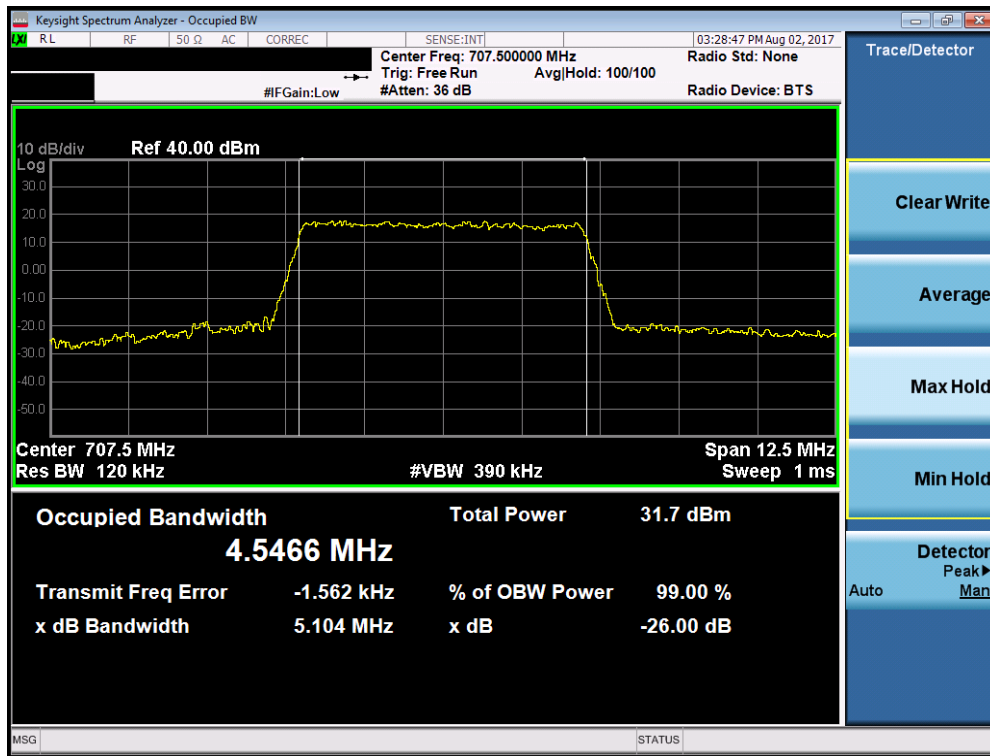
Plot 7-6. Occupied Bandwidth Plot (Band 12 – 5.0MHz 16-QAM – RB Size 25)
