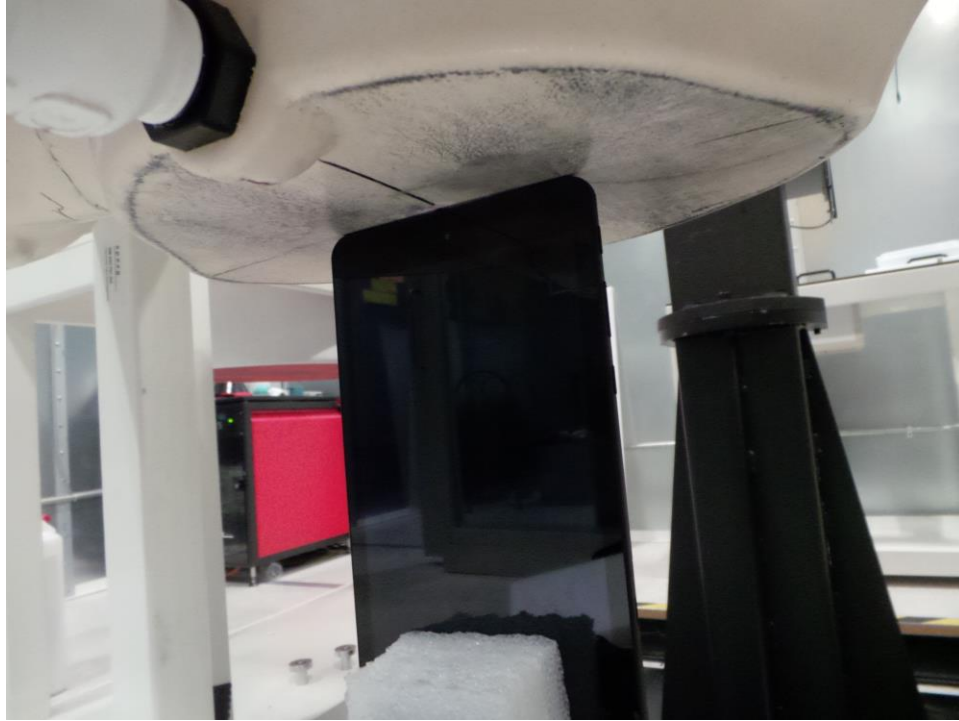
SAR Test Setup Photo 9 – Top Edge at 0 mm
