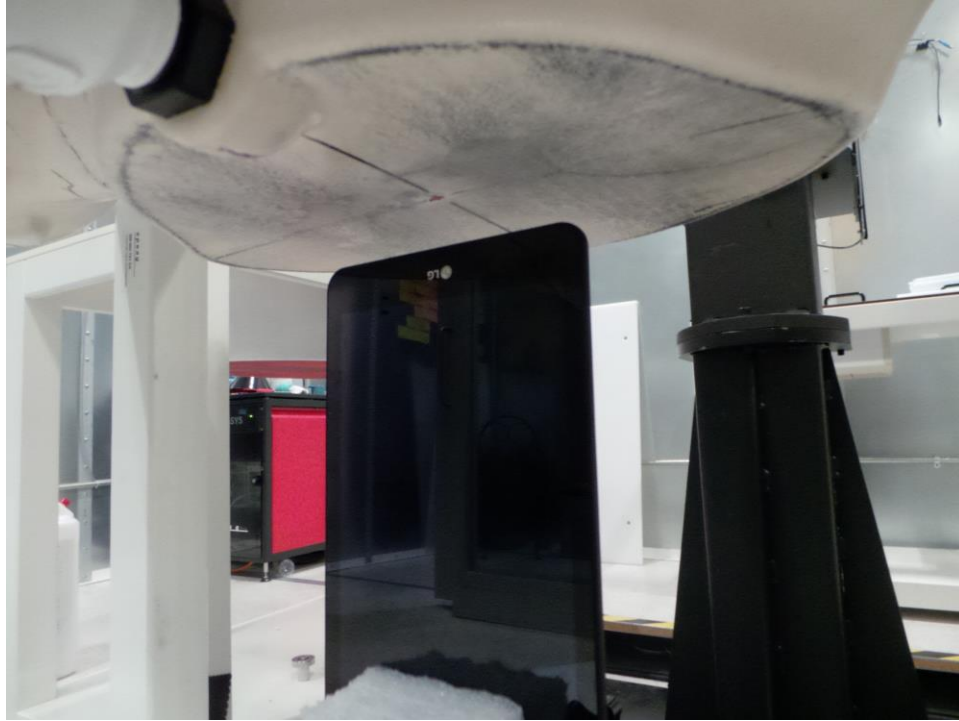
SAR Test Setup Photo 11 – Bottom Edge at 21 mm
