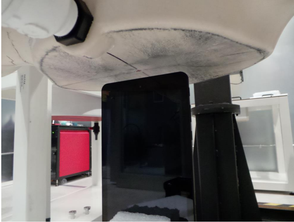
SAR Test Setup Photo 7 – Top Edge at 9 mm
