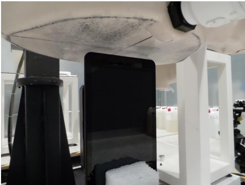
SAR Test Setup Photo 8 – Top Edge at 9 mm with Sound Pack
