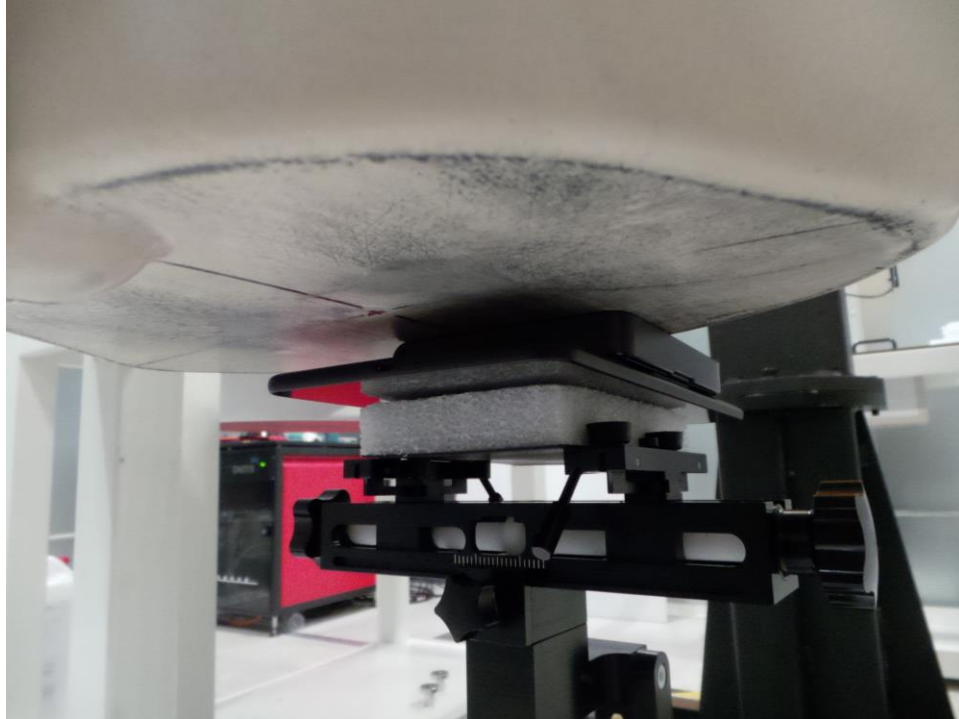
SAR Test Setup Photo 5 – Back Side at 0 mm with Sound Pack for Main Bands
