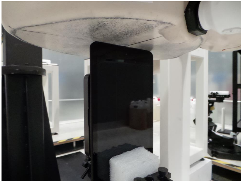
SAR Test Setup Photo 10 – Top Edge at 0 mm with Sound Pack
