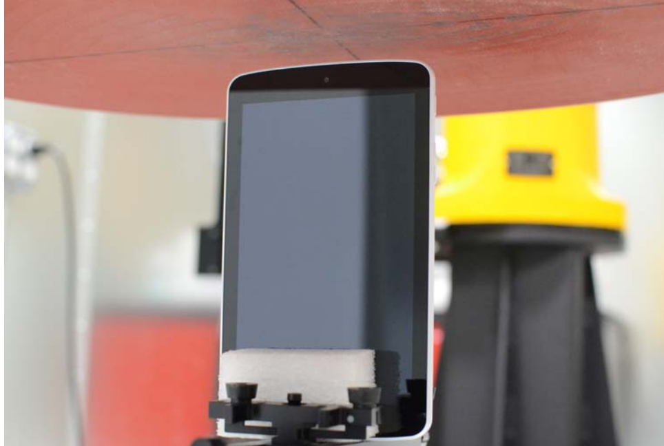
SAR Test Setup Photo 3: Top Edge at 1.6 cm
