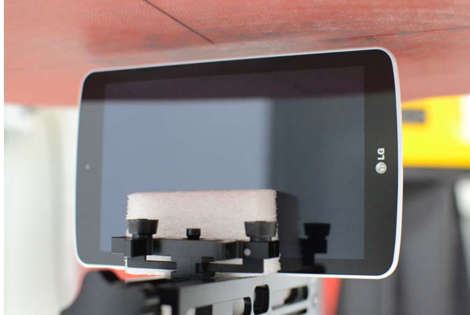
SAR Test Setup Photo 5: Right Edge at 0.5 cm
