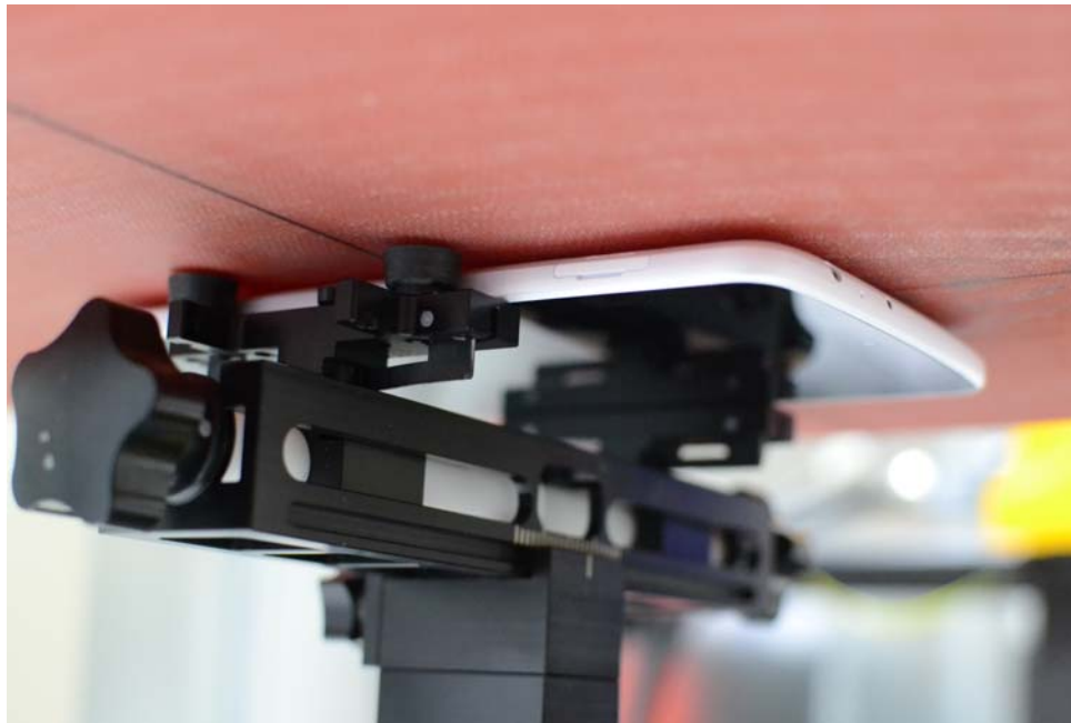
SAR Test Setup Photo 2: Back Side at 0.0 cm
