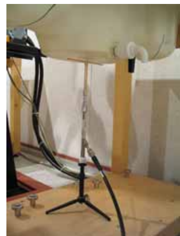
Photo of the dipole Antenna
