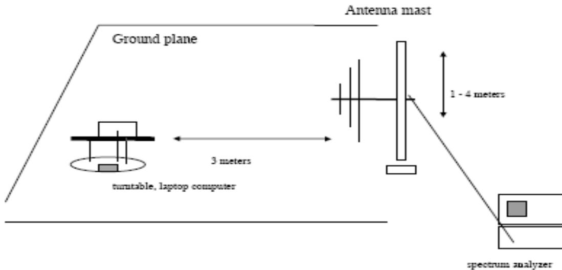
Test Procedures: Radiated emissions were measured according to ANSI C63.10.
