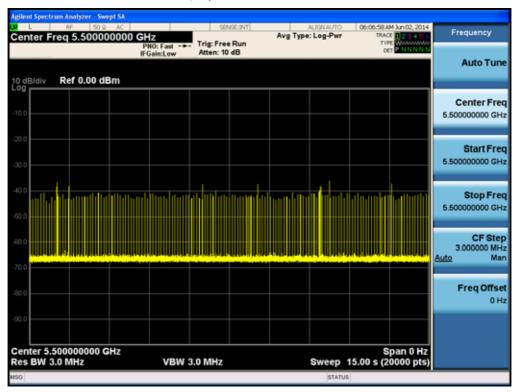
Time Display, WLAN Channel Traffic (Streaming Video)
