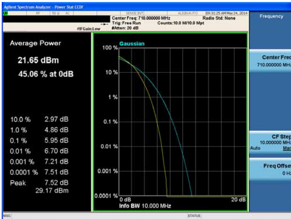
BAND 17. Peak to Average Ratio Plot (10M BW Ch.23790 16QAM RB 50)
