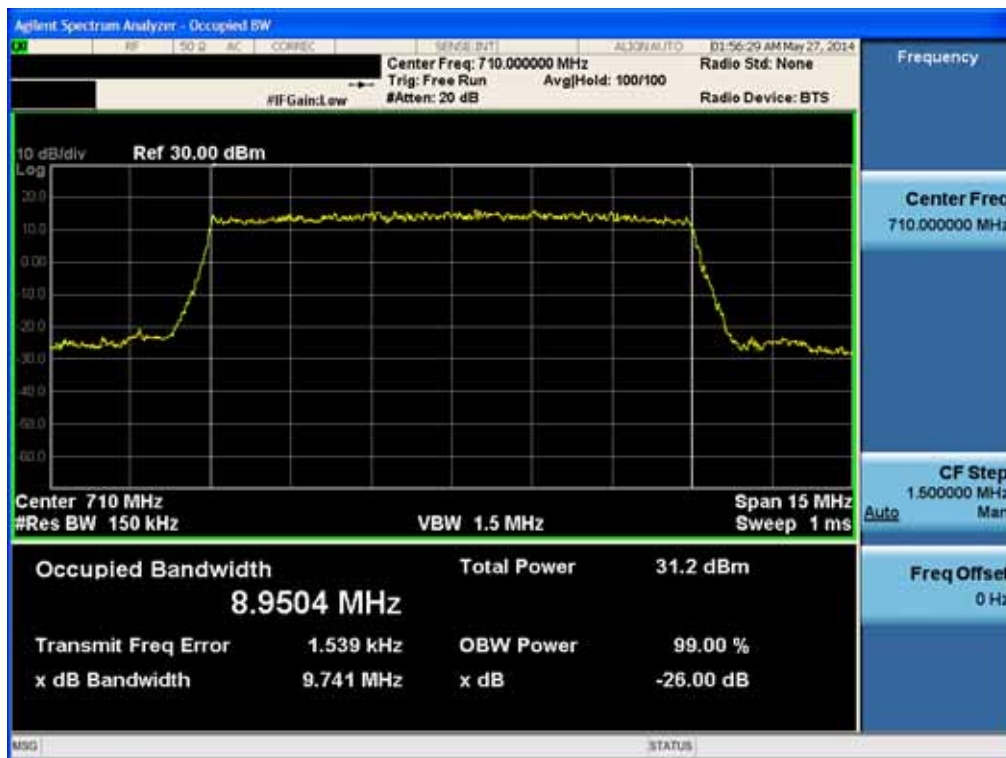
BAND 17. Occpied Bandwidth Plot (10M BW Ch.23790 QPSK RB 50)
