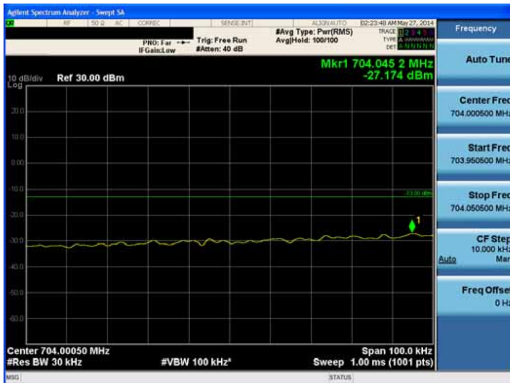
BAND 17. Lower Band Edge Plot (5M BW Ch.23755 QPSK RB 25) -2
