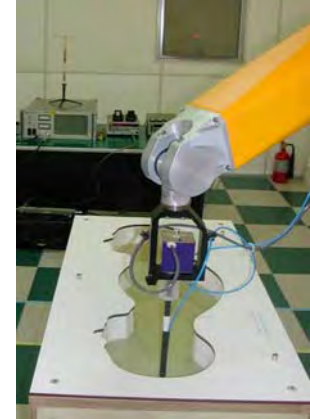
Figure 4.3 Photograph of the probe and the Phantom
