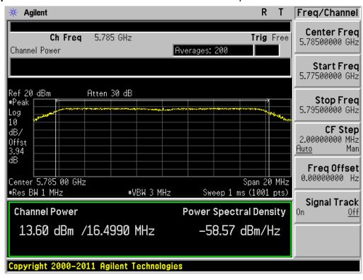
Peak Output Power Test Mode: 802.11a & 6Mbps & 5825MHz
