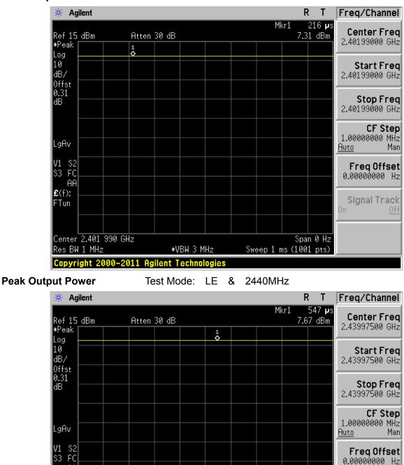
Peak Output Power Test Mode: LE & 2402MHz
