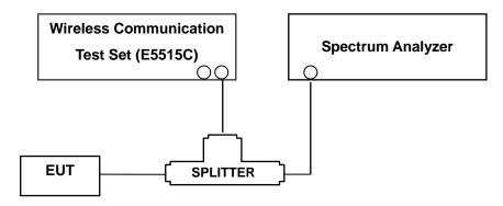
(Configuration of conducted Emission measurement)
