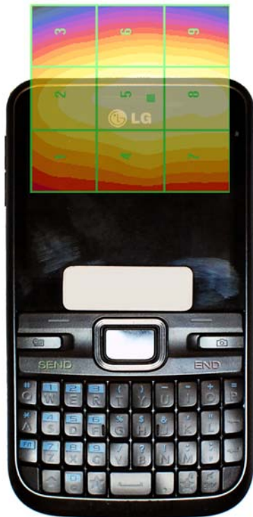
Figure 17-4 E-Field WD Scan overlay
