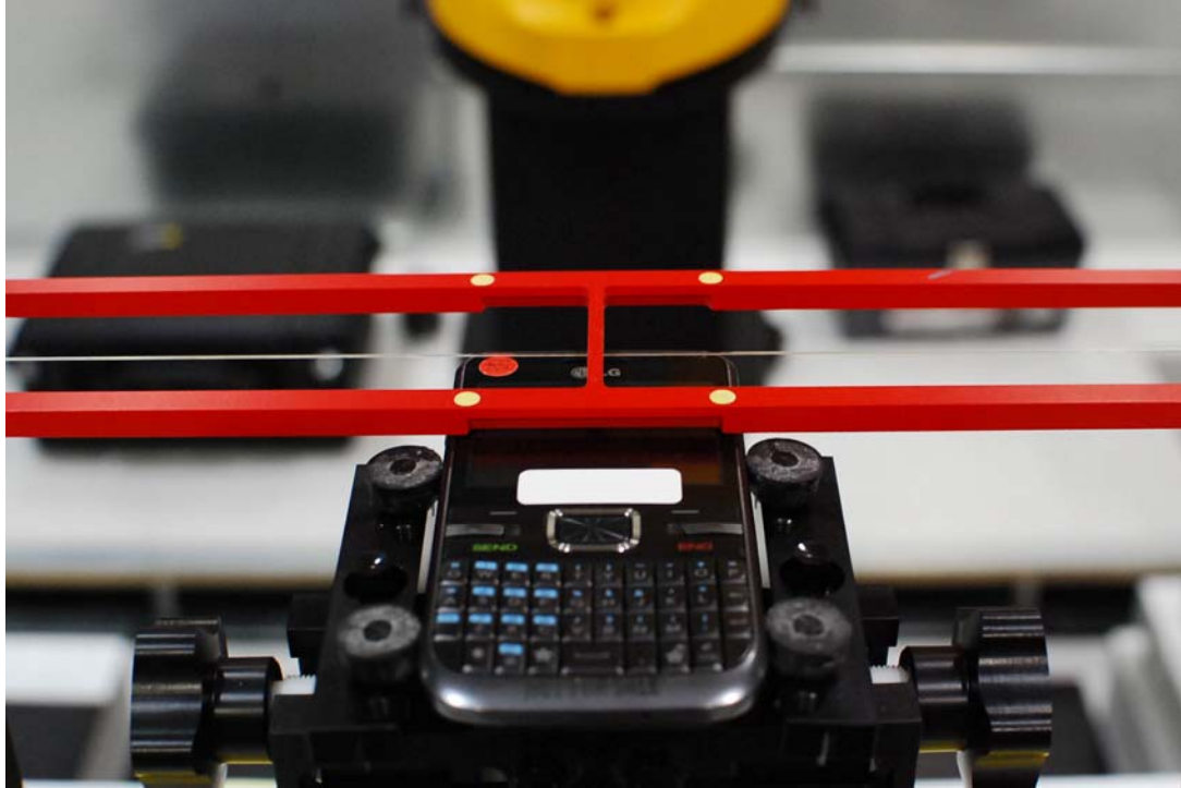
Figure 17-1 Ear Reference Point HAC Phantom Alignment
