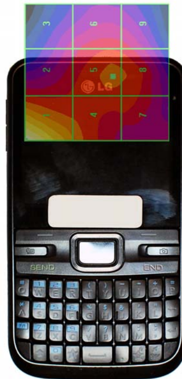
Figure 17-5 H-Field WD Scan overlay
