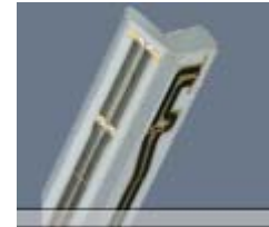
Figure 5-1 E-field Free-space Probe
