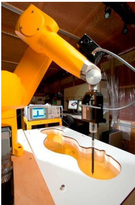
Figure 3-2 SAR Measurement System
