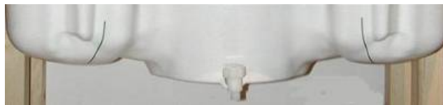
Figure 7-2 SAM Twin Phantom Shell
