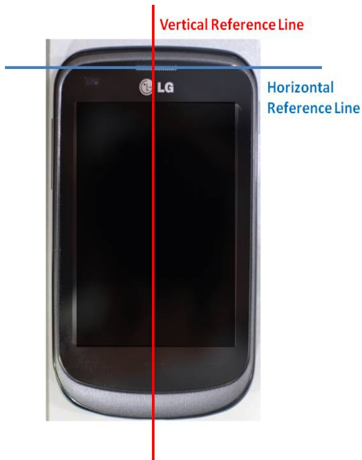
SAR Test Setup Photo 6 - Vertical and Horizontal Reference Lines
