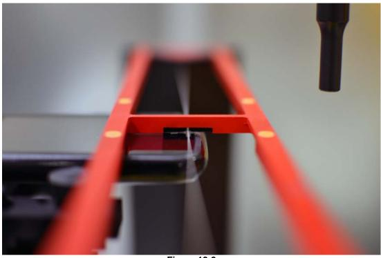
Figure 18-2 HAC Phantom Plane Alignment
