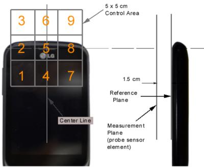
Figure 18-3 5x5 Scan grid above WD
