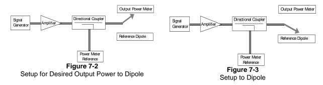
Using this setup configuration, the signal generator was adjusted for the desired output power (100mW) at a specified frequency. The reference power from the coupled port of the directional coupler is recorded. Next, the output cable is connected to the reference dipole, as shown in Figure 7-3.
