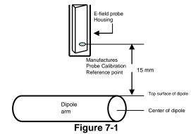
Separation Distance from Dipole to Field Probe
