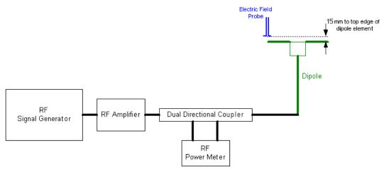
Figure 7-8 System Check Setup
