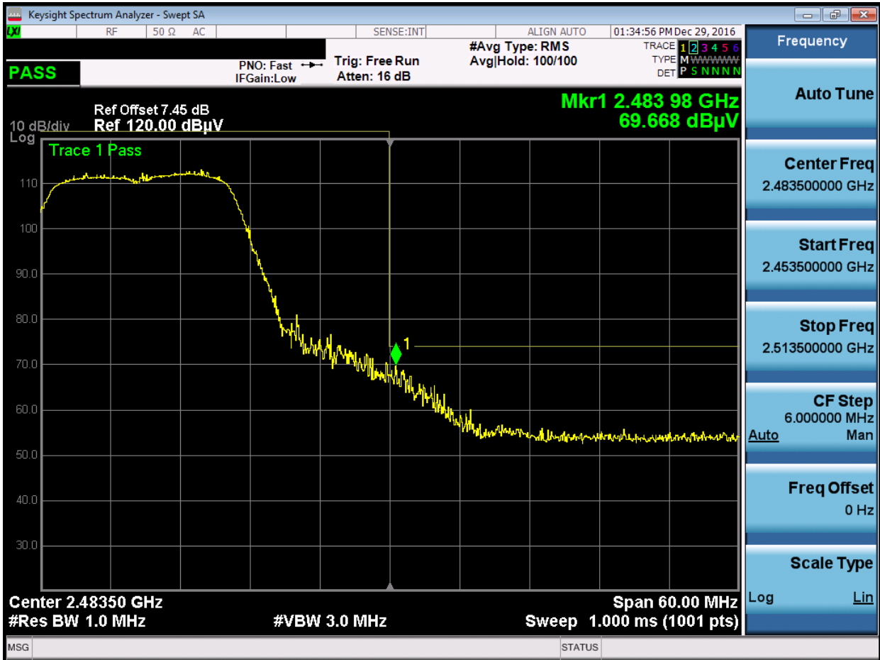
Plot 7-12. Radiated Restricted Upper Band Edge Measurement (Peak)
