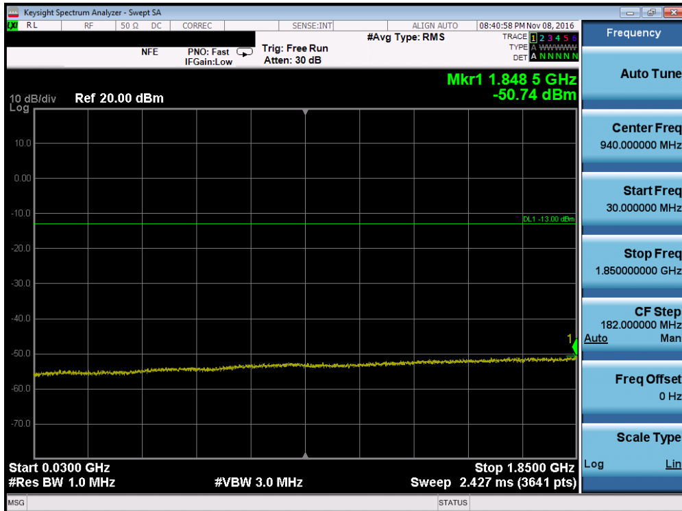
Plot 7-74. Conducted Spurious Plot (Band 2 – 3.0MHz QPSK – RB Size 1, RB Offset 0 – High Channel)
