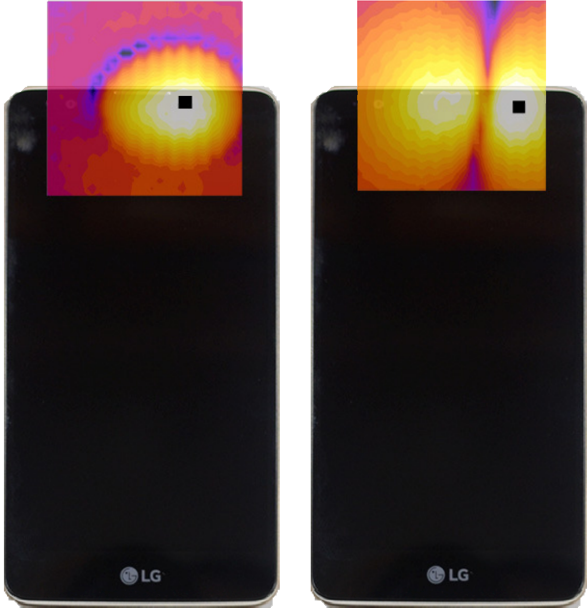
Figure 14-3 T-Coil Scan Overlay Magnetic Field Distributions
