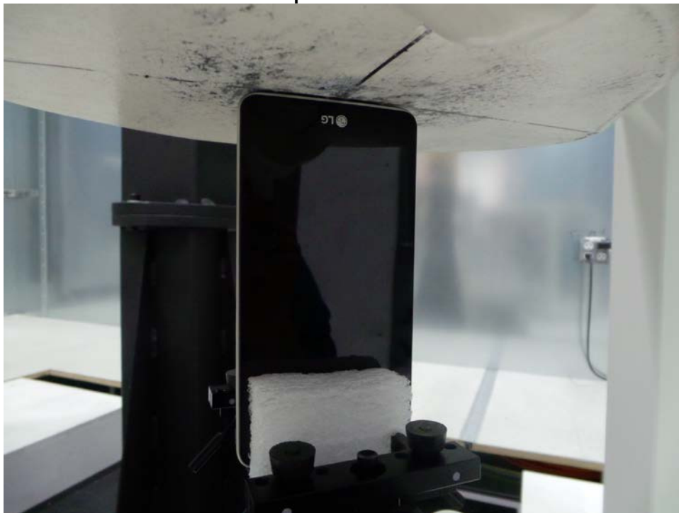
SAR Test Setup Photo 8 – Bottom at 0mm
