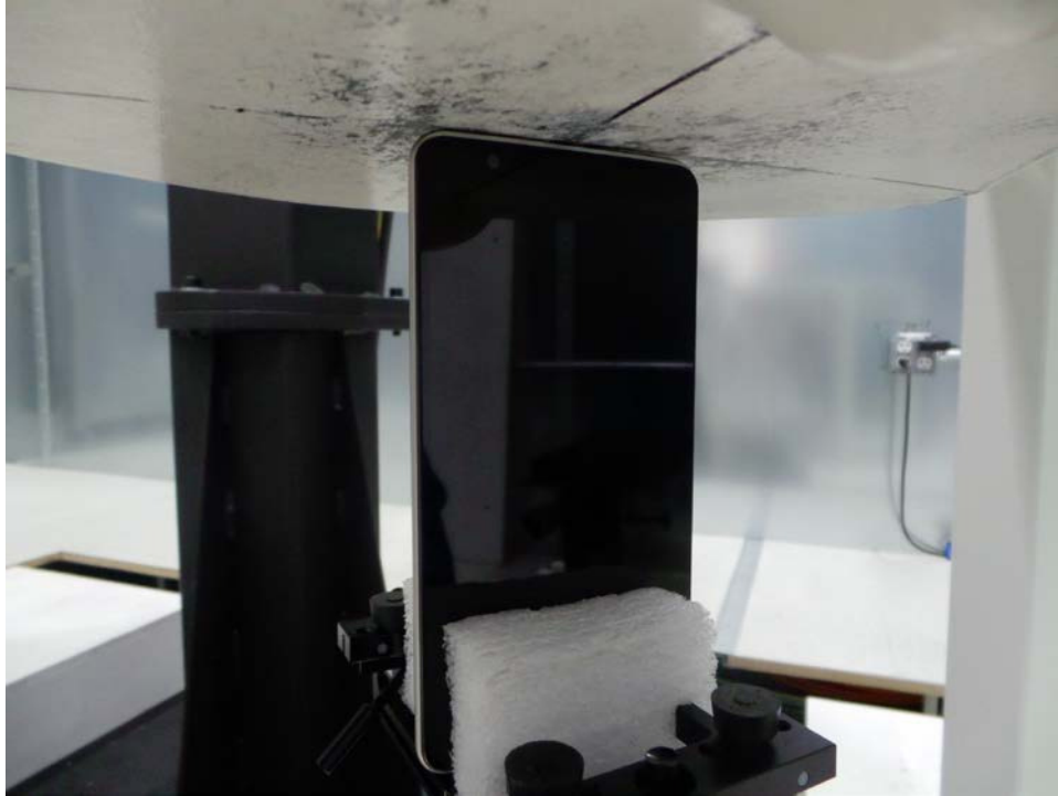
SAR Test Setup Photo 9 - Top at 0mm
