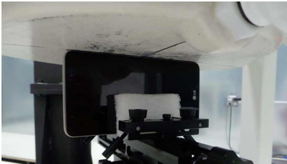
SAR Test Setup Photo 10 - Right at 0mm
