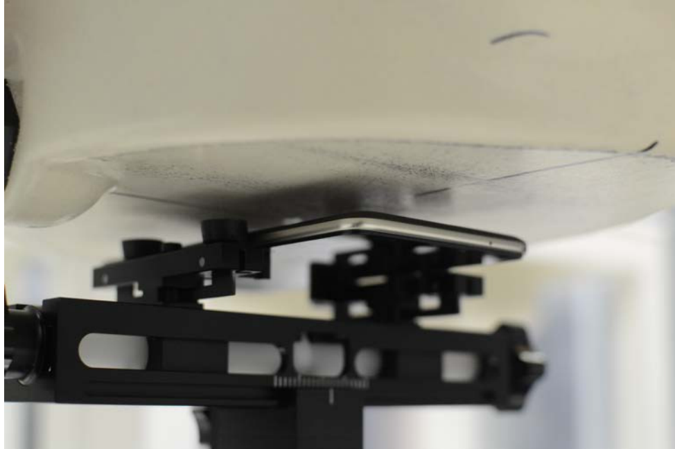
SAR Test Setup Photo 5 – Back at 10mm
