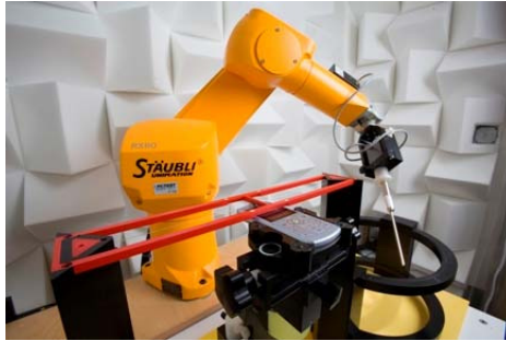
Figure 5-3 SPEAG Robotic System
