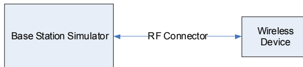
Figure 9-1 Power Measurement Setup
