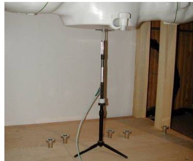
Figure 10-2 System Verification Setup Photo
