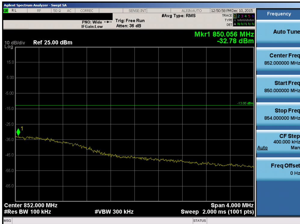
Plot 7-90. Upper Extended Band Edge Plot (Band 5 – Band 5 – 3.0MHz QPSK – RB Size 15)
