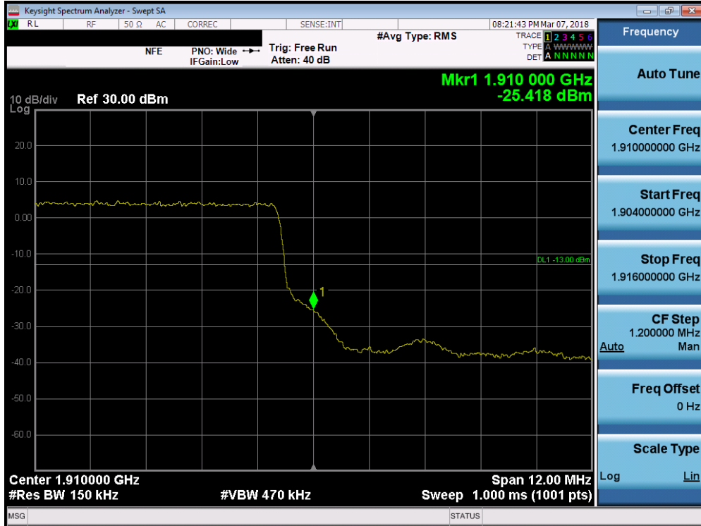
Plot 7-222. Upper Band Edge Plot (Band 2 - 15.0MHz QPSK - Full RB Configuration)
