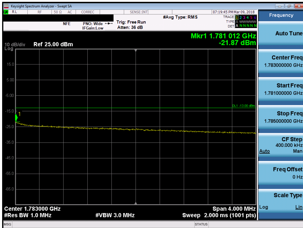
Plot 7-191. Upper Extended Band Edge Plot (Band 66 - 10.0MHz QPSK - Full RB Configuration)
