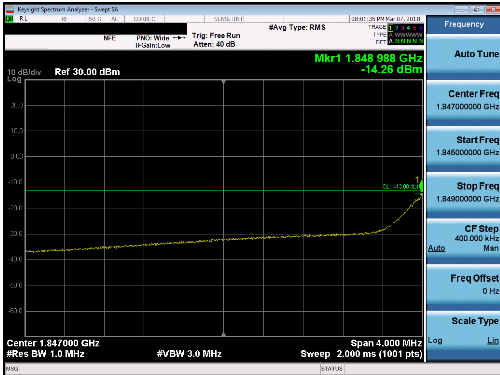
Plot 7-213. Lower Extended Band Edge Plot (Band 2 - 5.0MHz QPSK - Full RB Configuration)
