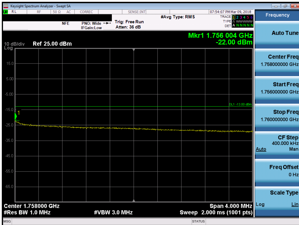
Plot 7-189. Upper Extended Band Edge Plot (Band 4 - 10.0MHz QPSK - Full RB Configuration)
