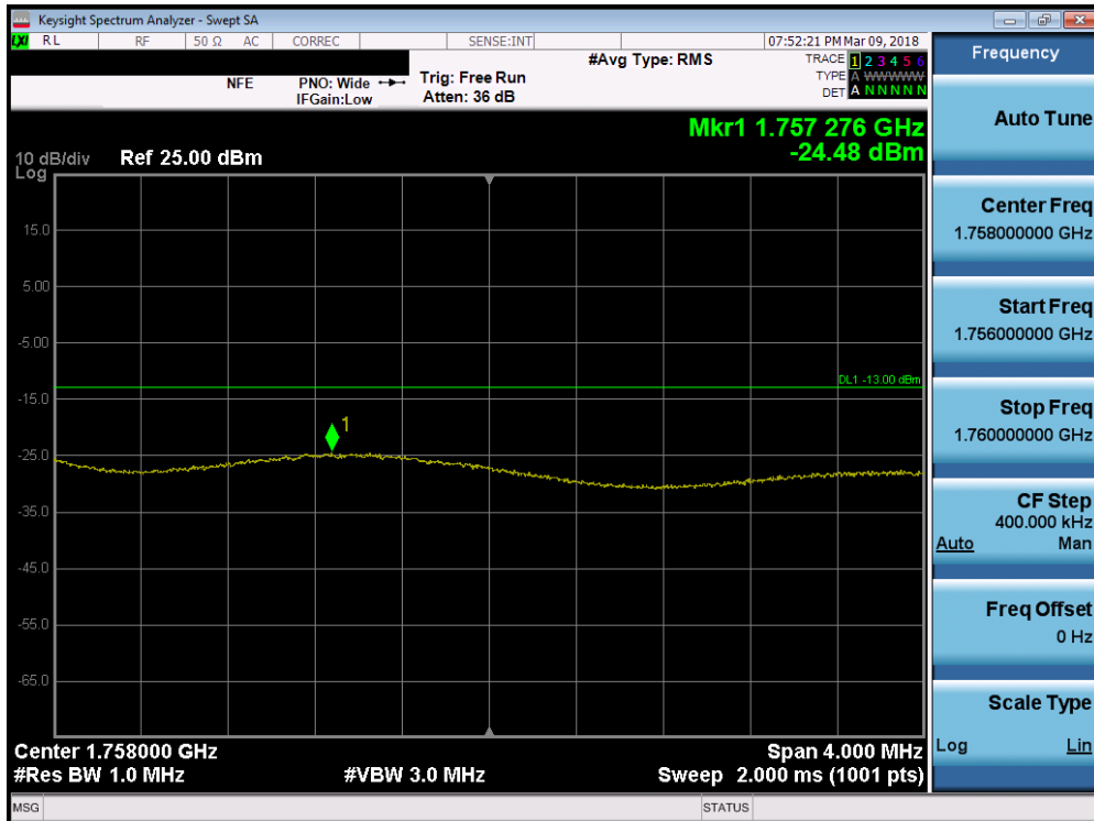
Plot 7-195. Upper Extended Band Edge Plot (Band 4 - 15.0MHz QPSK - Full RB Configuration)
