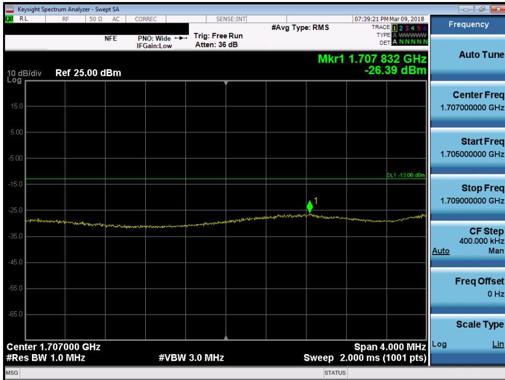
Plot 7-193. Lower Extended Band Edge Plot (Band 66/4 - 15.0MHz QPSK - Full RB Configuration)
