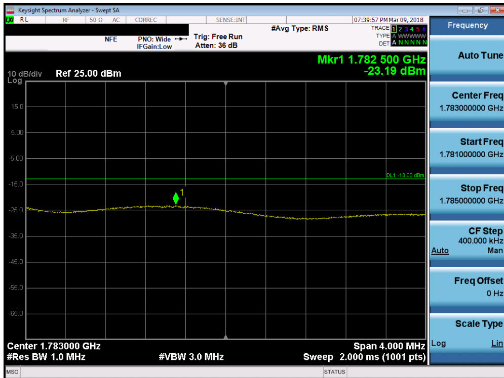
Plot 7-197. Upper Extended Band Edge Plot (Band 66 - 15.0MHz QPSK - Full RB Configuration)
