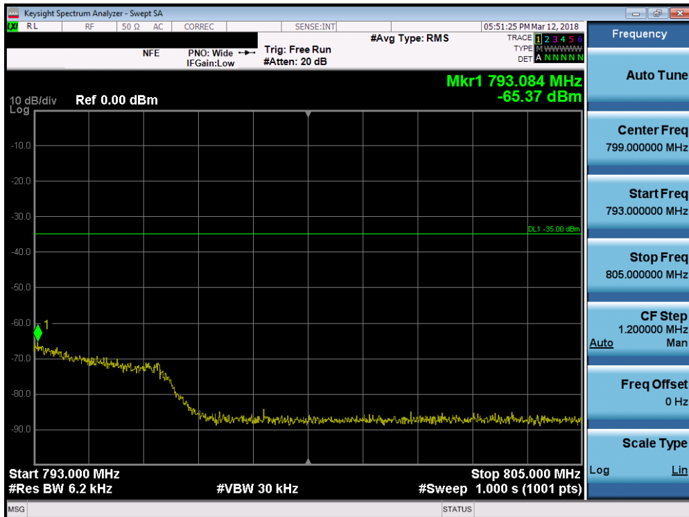
Plot 7-155. Upper Emission Mask Edge Plot (Band 13 - 5.0MHz QPSK - Full RB Configuration)
