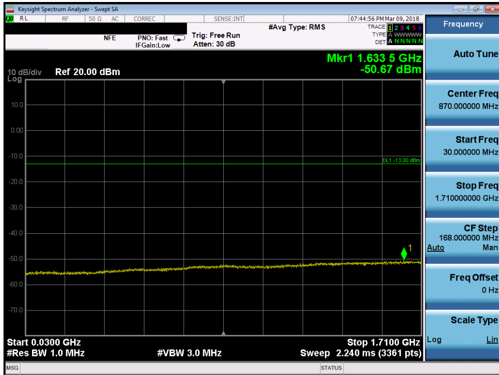
Plot 7-124. Conducted Spurious Plot (Band 66/4 - 20.0MHz QPSK - RB Size 1, RB Offset 0 - High Channel)
