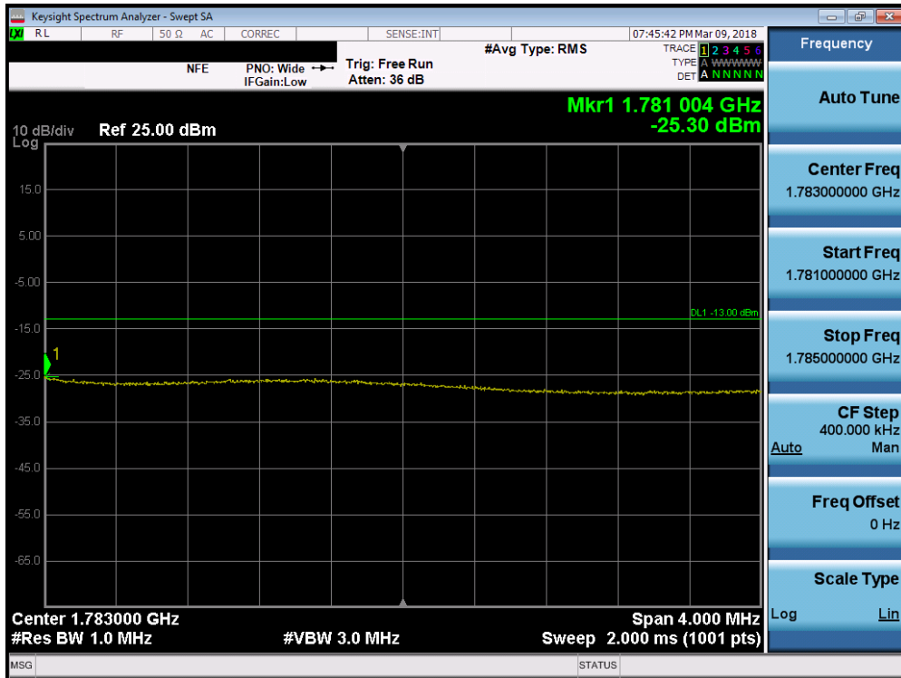
Plot 7-203. Upper Extended Band Edge Plot (Band 66 - 20.0MHz QPSK - Full RB Configuration)
