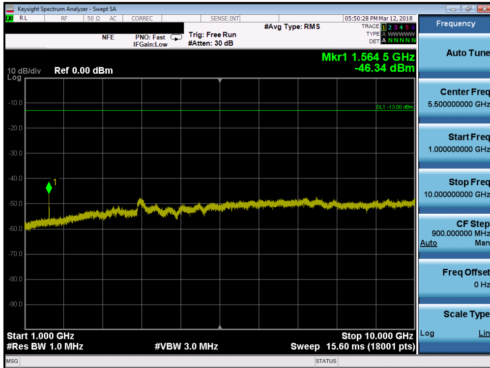
Plot 7-105. Conducted Spurious Plot (Band 13 - 5.0MHz QPSK - RB Size 1, RB Offset 0 - High Channel)
