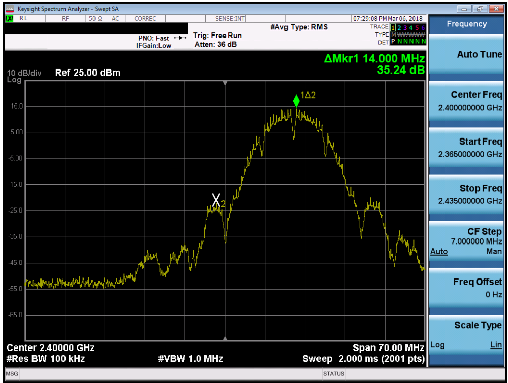
Plot 7-19. Band Edge Plot (802.11b – Ch. 1)
