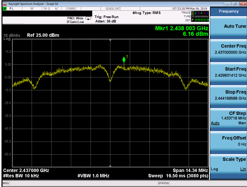
Plot 7-11. Power Spectral Density Plot (802.11b – Ch. 6)
