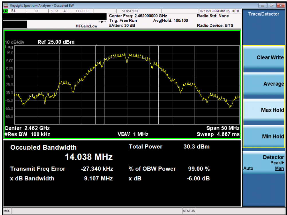
Plot 7-3. 6dB Bandwidth Plot (802.11b – Ch. 11)
