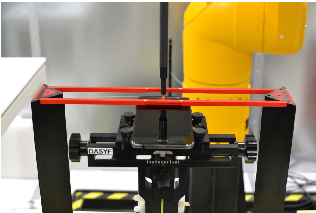
Figure 17-1 Ear Reference Point HAC Phantom Alignment
