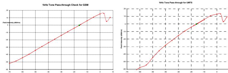
This model was verified to be within the linear region for ABM1 measurements at -16 dBm0 for GSM, and UMTS. This measurement was taken in the axial configuration above the maximum location.
