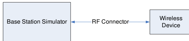
Figure 9-1 Power Measurement Setup
