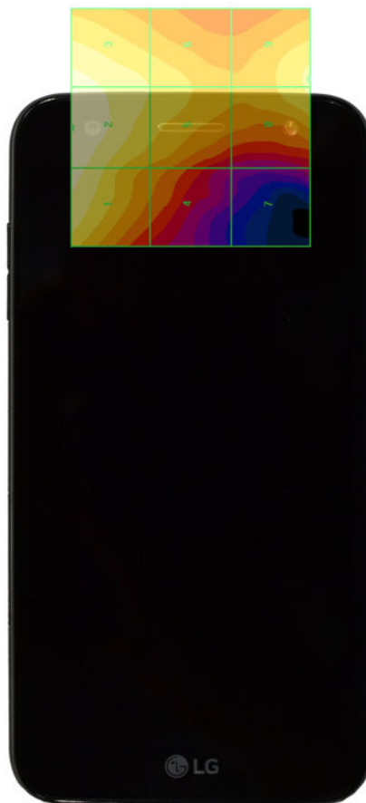
Figure 17-4 E-Field WD Scan overlay
