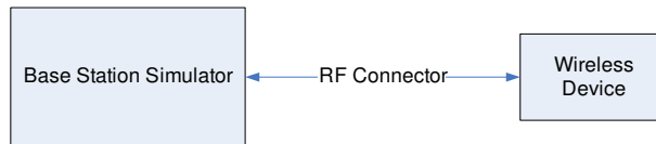
Figure 9-2 Power Measurement Setup
