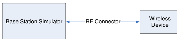
Figure 9-1 Power Measurement Setup
