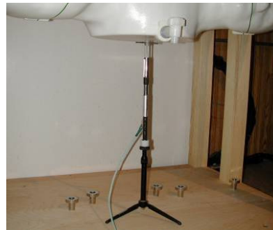
Figure 10-2 System Verification Setup Photo
