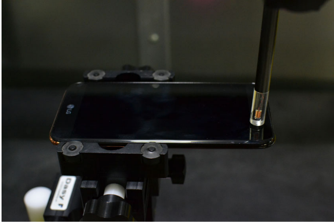
Figure 13-1 Test Setup for Wireless Device
